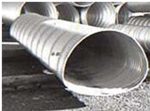
Figure 9. Example of a metal pipe arch culvert.
